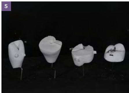
FIGURE 5: Common milling faults from left to right: chipped screw hole channel caused by fractured burr, complete failure of molar restoration caused by fractured disc, holes within the occlusal surface, restoration designed to minimum thickness followed by inaccurate CNC calculation
