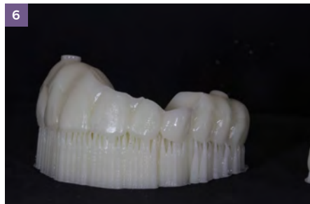
FIGURE 6: Failed 3D-printed bridge
