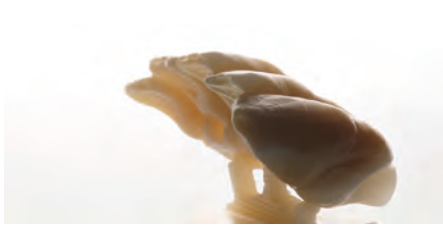
FIGURES 19-21: The zirconia restoration sintered with the Speed program in the Zirkonofen Turbo
