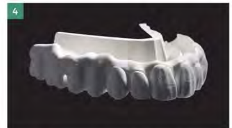
FIGURE 4: The result in the chalk stage before sintering
