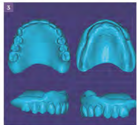
FIGURE 3: STL of the denture imported to design software
