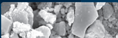
Clearly visible in the SEM image: The bead structure of OMNICHROMA compared to conventionally crushed particles.
