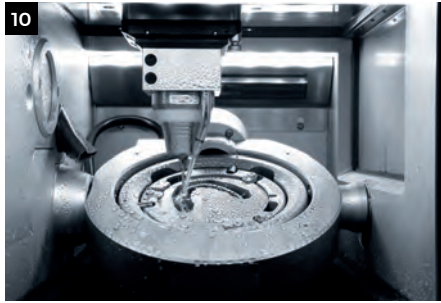
FIGURES 10 and 11: High-quality bars require a smooth surface and extreme precision in the milling of implant connections and geometries
