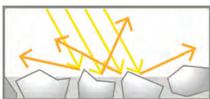
Figure 2: Traditional irregular particles reflect light randomly resulting in a dull matt appearance
