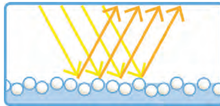
Figure 1: Tokuyama spherical particles reflect light uniformly for a perfect shine
