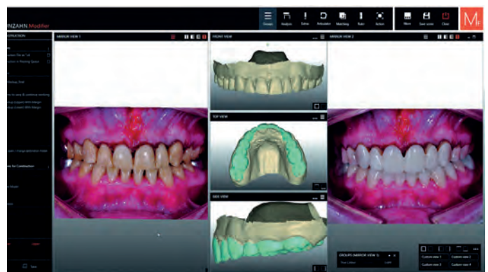
Digital planning of the gingivectomy in the Zirkonzahn.Modifier software showing definition of the new occlusion and design of the temporary mock-up which is the key tool for checking and reproducing all workflow steps up to the final restoration
