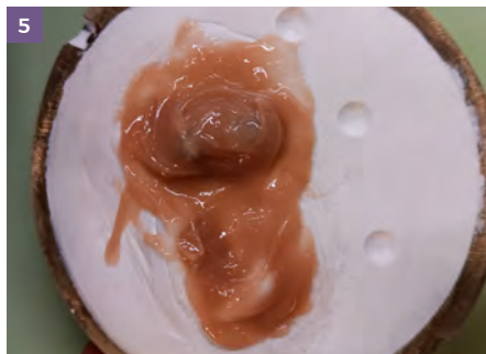
FIGURES 5 and 6: A small proportion of the base silicone is then placed in the mould before the cushion is placed on top of it
