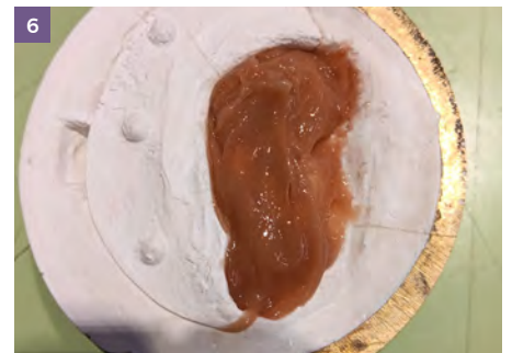
FIGURES 5 and 6: A small proportion of the base silicone is then placed in the mould before the cushion is placed on top of it
