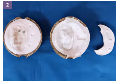
FIGURE 2: A small 'cushion' of plaster is added to the invested wax pattern
