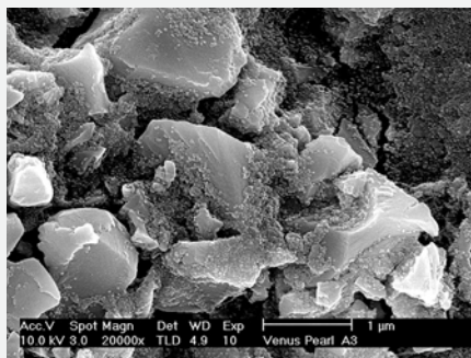
FIGURE 2: SEM of irregular filler composite material
