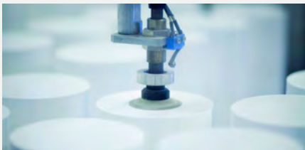
FIGURE 2: Zirconia blanks production. Each production batch is accurately checked after every step, via specific tests and measurements to control hardness, dimensions, density, milling, colour, translucency as well as the materials' shrinkage factor, using close-tolerance instruments
