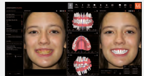
FIGURE 1: The lecture will focus on a complex restoration 100% digitally created, starting from diagnostic analysis and complete 3D virtual reproduction of the patient's oral and extraoral anatomy without loss in information: initial situation (left) and first digital tooth setup (right)
